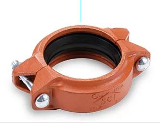
Figure 65LFTRI & 66LFTRI Lightweight Flexible couplings are designed for use in piping systems where flexibility is desired. They allow for pipe movement caused by seismic action and thermal variations, and will also attenuate noise and vibration transmitted through the piping system.
